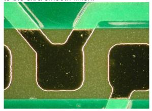
Poor bondability Note that there is more of a gold color when photographed due to the non-smooth / coarse plating.
